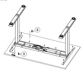
**Step 11:** Ensure that the cables are placed properly and plug the cables into the control box. Use the cable clamps to fasten the cables for the control box.
