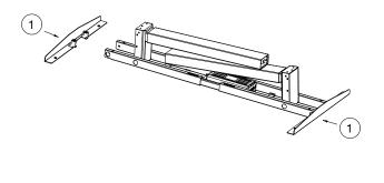
Step 4: Ad 8 M6x10 hexagon screw through the frame into the motor house of the columns. Tighten the screws.
