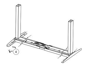
**Step 5:** Ad the feet on to the columns and fasten each with 2 M8x14 mm screws. Tighten the screws.
