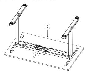
Step 10: Tighten all 8 screws in the frame.
