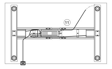
**Step 6-7:** Place the frame on the table top. Pull out the frame and make sure that it is placed 60 mm from the edge, if you have a 1200-1800 mm table, and 100 mm form the edge if you have a 2000 mm table. Make sure that the connection rails are centered.
