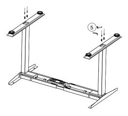
**Step 8-9:** Mount the frame to the table top with 7 5x20 mm wood screws and the handset with 2 5x20 mm wood screws. Tighten the screws.
